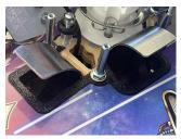
Now reinstall the rubber on the posts and reattach the bottom plastic (don't forget to put those spacers back in and be careful when you tighten down the small pop bumper screws, it's easy to overtighten them and pull them right through the plastic). Finally, reinstall the top plastic and the extra post screw.
