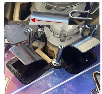
protector slide in between. Adjust the position of the tab up or down until the top lip sits cleanly against the wood and the hole for the post aligns with the hole in the protector, then slowly relax your pull and let the scoop metal pinch the rubber against the wood, holding it in place. Reinstall the posts and adjust until it fits properly and fills in the outlines.
