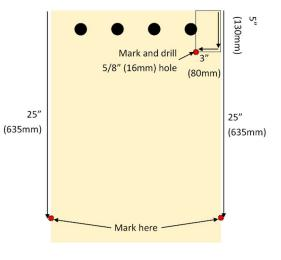
Second, measure and mark the point halfway down each side of the cabinet, about 25" (635mm).
