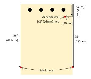
Second, measure and mark the point halfway down each side of the cabinet, about 25" (635mm).
